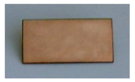
Figure 5. A Thick Application of Enamel Flux
