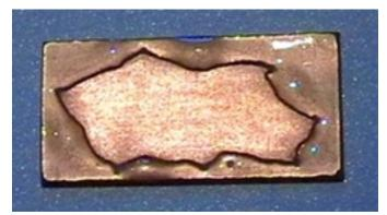
Figure A5. Unsatisfactory Bonding of Enamel to Metal
