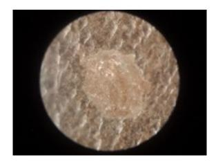
Figure 10. Magnified View of Pit Inadequately Repaired, (1mm Field of View)
